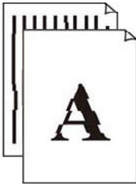
Lines Are Misaligned/Distorted
