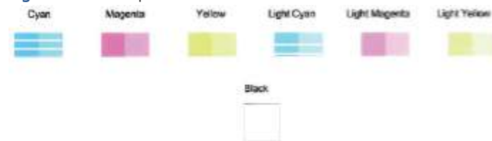
Figure 9-2 Example of color blocks with defects
