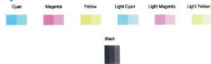
Figure 9-2 Example of color blocks with defects
