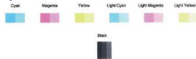
Figure 9-2 Example of color blocks with defects
