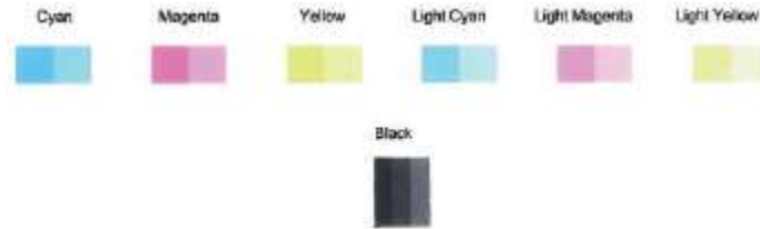
Figure 9-2 Example of color blocks with defects
